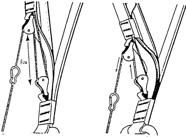
Normal flight may be resumed immediately, simply releasing the stirrup smoothly allows the risers to return to their standard trim position, it is possible to react flexibly with this system, even in turbulent conditions.
